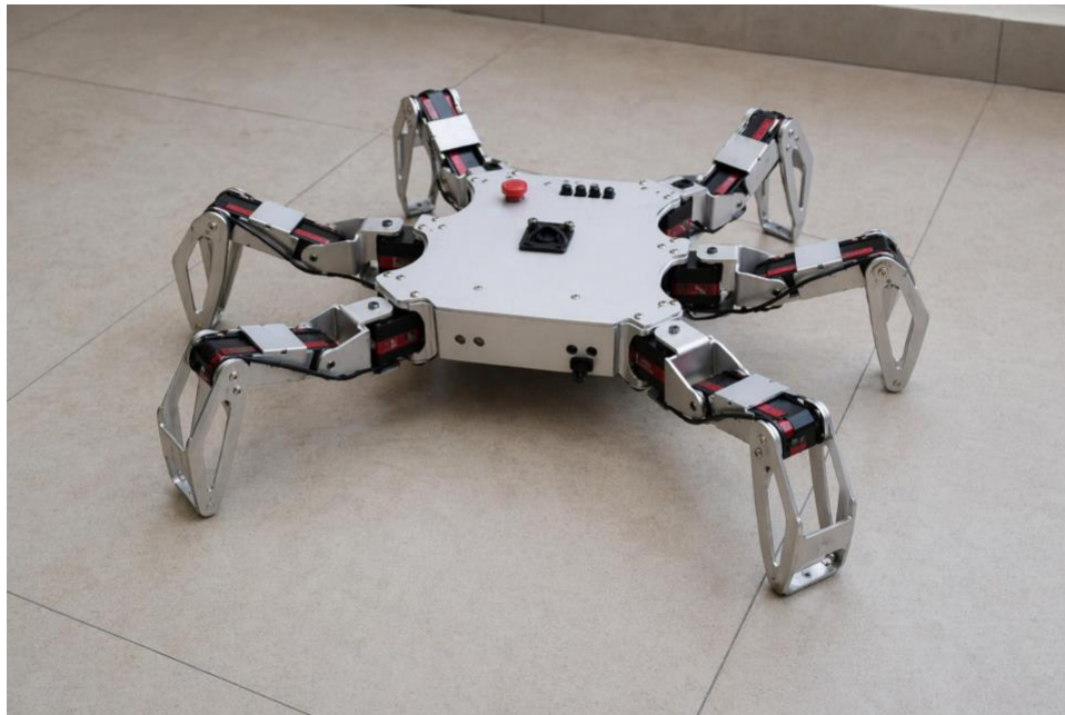
Figure 1 — HexaPod assembly, 18-DOF configuration
